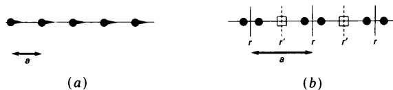
Fig. 2. Patterns illustrating the two possible 1D space groups. (a) Space group P1 . (b) Space group Pr ; r and r' are 'reflections' which are the 1D equivalent of mirrors, inversion centres or twofold axes.
